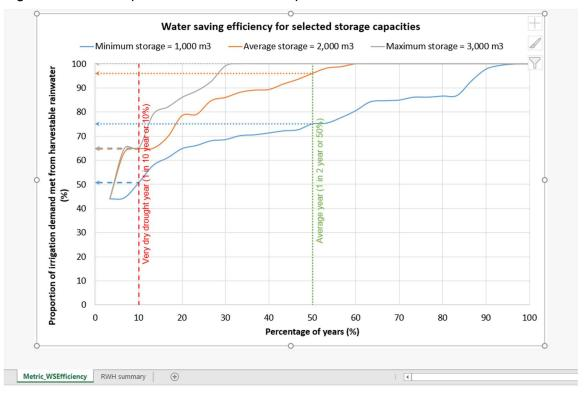
This figure shows the relationship between the percentage of irrigation demand met from the harvestable rainwater (%) and the percentage of years (%). As with the irrigation deficit metric, the data are based on 30 years historical weather and for three reservoir capacities.
