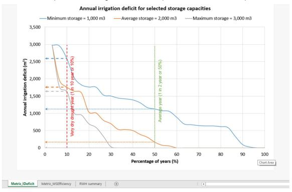
This figure shows the cumulative probability (percentage of years) for the annual irrigation deficit metric based on 30 years of historical weather data, for three reservoir capacities (1,000, 2,000 and 3,000 m³). The minimum and maximum capacities were defined on the Site data entry sheet.
