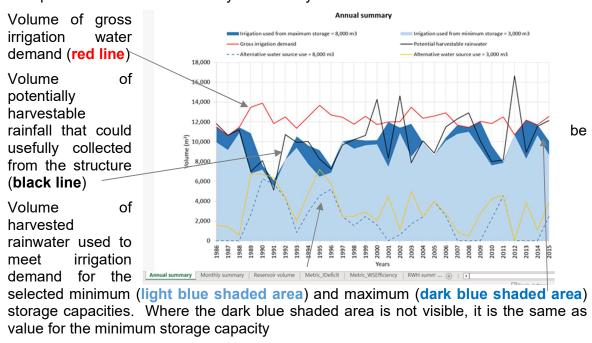
Volume of water used from the alternative source due to insufficient availability of harvested rainfall in the selected minimum (yellow line) and maximum (dashed blue line) capacity reservoir.
